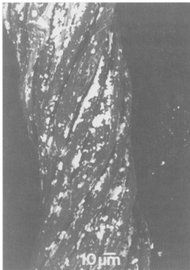
FIG. 2. A backscattered electron image of an oil/clay treated yarn washed with unbuilt, liquid detergent at 27 C.
